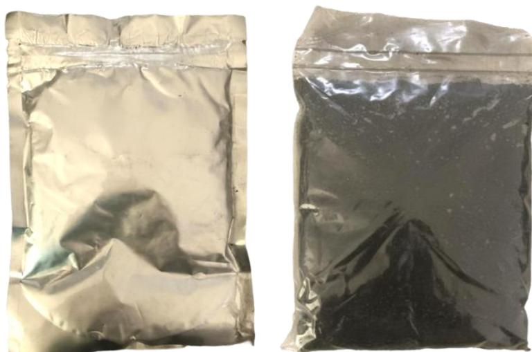
**Figure 3.** Sample of a Soil-Charcoal-Based Solid Biofertilizer Formulation Packaged in Aluminum Foil and PPE Plastic and Stored Under Ambient and Air-Conditioned Rooms
