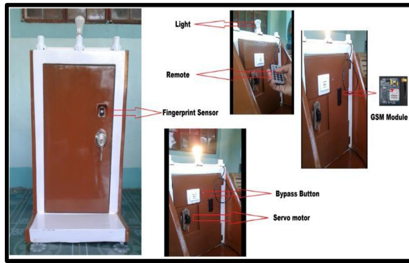
Figure 9. The Developed Device
