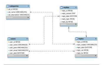
**Figure 4.** Database Schema of the Web-Based Information System
