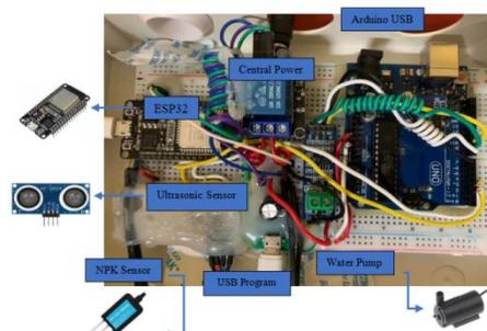
**Figure 3.** *Arduino-Based Nutrient Analysis and Deficiency Tracker.*
