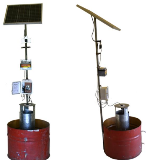
Figure 8. The Prototype Assembly of the Developed Integrated Solar-Powered Wireless IoT-Based Water Level Monitoring Embedded System (Front, Side Views)
